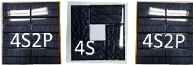
Fig. 7. Final assembly of the solar panels.
