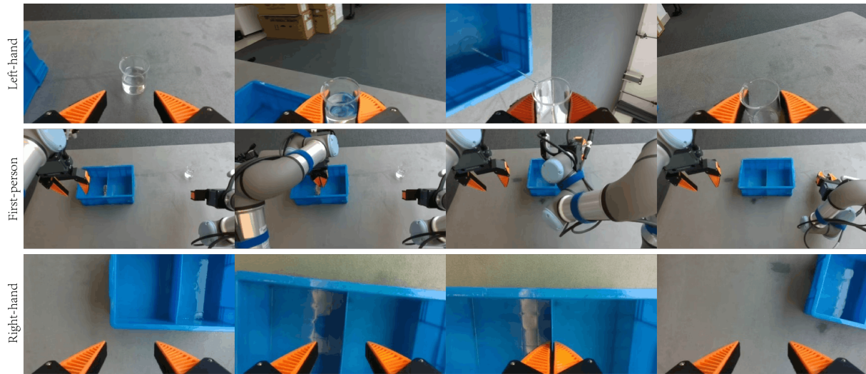
Fig. 4. Three perspectives of pouring the water in the beaker into the tank. Sequence of robot actions from left to right: initial pose, grasp and move the sink with the left claw, grasp the beaker to pour water into the sink with the right claw, and return to the neural position
