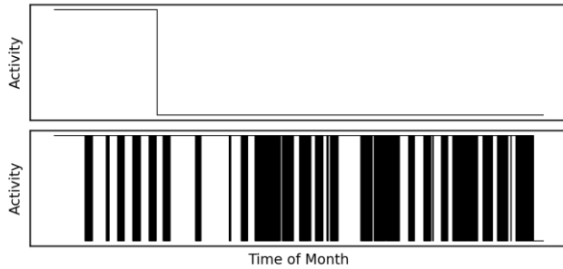
Figure 2. Alarm dynamics illustration for a 1-month period in an educational building: low (top), high (bottom) activity air flow alarm
