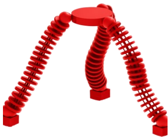
Figure 1 Hybrid parallel soft–rigid robotic system with three continuum actuators linked to a rigid upper platform via free joints, adapted from Nuelle et al. [33].
