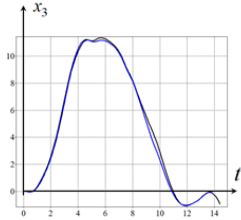
Fig. 3. Graphic of variable x_3 at movement on the circle. Blue line is real object, black line is identification model
