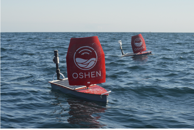
Fig. 1. C-Star autonomous surface vehicle (ASV) platform context for the flow-aware waypointing problem considered in this paper.
