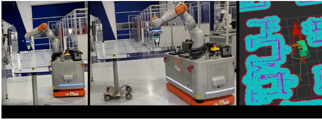
Fig. 5. KUKA KMR hardware experiment. (a) Static-footprint path planned close to the table obstacle. (b) Proposed dynamic footprint accounting for the extended arm during obstacle avoidance. (c) RViz visualisation of the costmap and planned trajectories.
