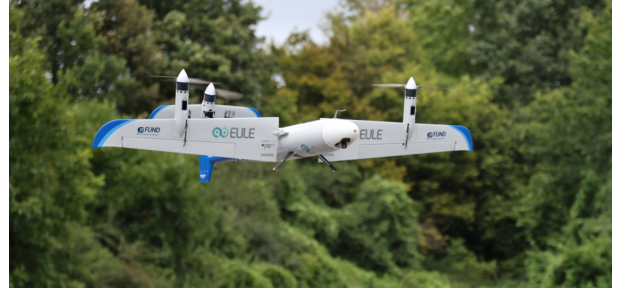
Fig. 5: Tilt-wing UAV: TW-Neo in multirotor mode
