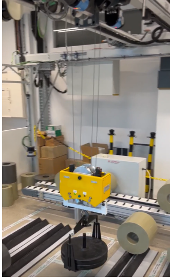
(c) Real overhead crane (loaded case)
