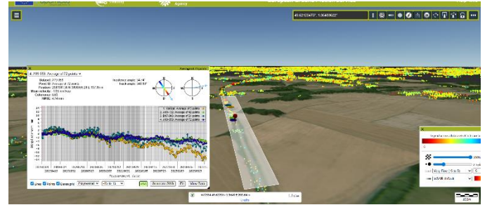
Fig. 4. Example of InSAR time-series image showing line-of-sight displacements along a railway corridor.
