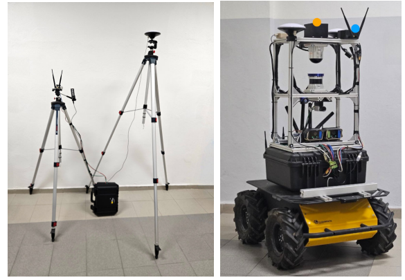
Fig. 3. On the left, the base station with GNSS receiver and communication hardware. On the right, the wheeled robot Husky A200 with a GNSS receiver providing localization data and the communication hardware measuring signal strength. The orange disks show the location of the Mesh-FSK Flood communication receiver, and the blue dot shows the location of the Mesh-LTE receiver.
