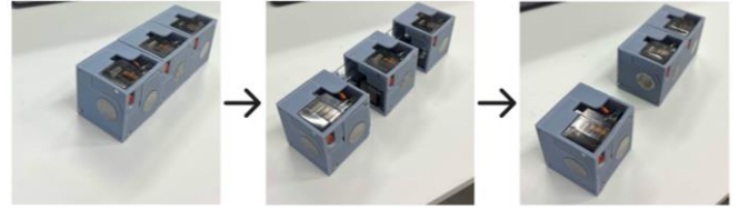
Fig. 9. Cooperative push displacement on physical hardware. Three modules in a line configuration: initial position (left), mid-displacement after two half-extensions (center), and full one-grid displacement after faces return to initial position (right). The reverse sequence performs the pull operation.
