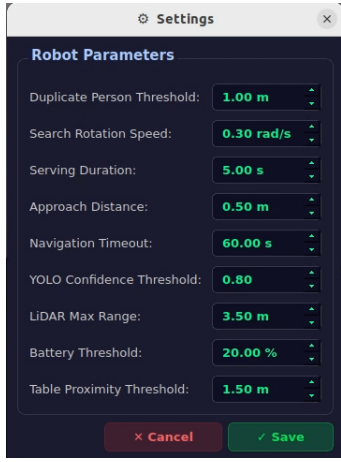
Fig. 5. PyQt5 desktop operator application used for wizard-based setup, live robot supervision, and runtime parameter tuning.
