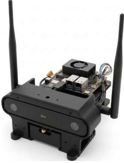
Fig. 1. Sensor suite used in the experiments.
