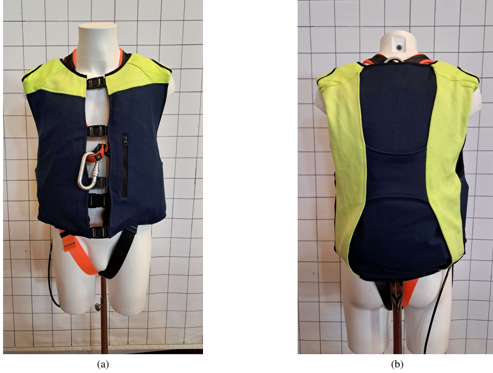
Fig. 1: A mannequin wearing the certified UNI EN 361:2003 harness and the deflated wearable airbag. (a) Front view. (b) Back view.
