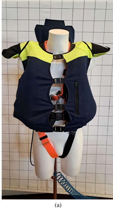
Fig. 2: A mannequin wearing the certified UNI EN 361:2003 harness and the inflated wearable airbag. (a) Front view. (b) Back view.
