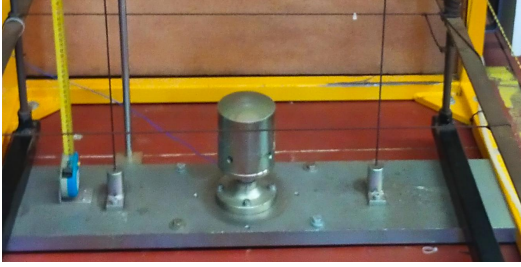
Fig. 6: The anvil and the load cell used for impact tests according to the EN1621-4 standard.
