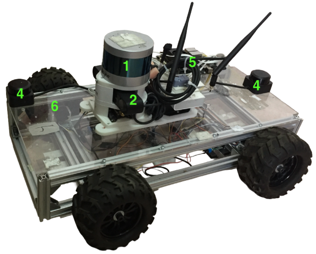
Fig. 2. Physical architecture of the developed skid-steer mobile robot, highlighting the placement of the computational units and sensory hardware.
