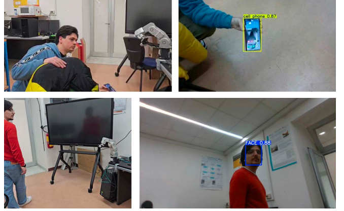
Fig. 2. Snaps of the object (top) and face (bottom) tracking experiment. Robot view and tracked object (right); external view (left).
