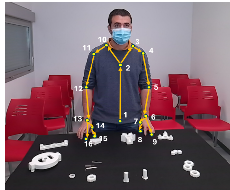
Fig. 1. Sample frame from the HA4M dataset. The operator stands behind a desk on which all assembly components are arranged. Skeleton joints are superimposed on the operator and numbered sequentially from 1 to 16.
