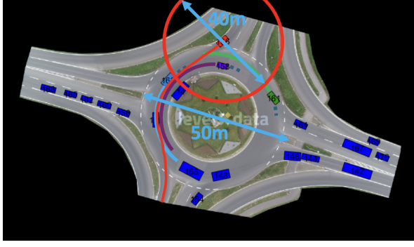
Fig. 4: Hypothesis on the road-users’ predicted trajectory. The vehicles follow a constant velocity model based on a data history of 400ms. The horizon of time of the prediction is 5 seconds. The trajectory of the IV (in red) is based on ELC trajectory and the obstacle vehicles are following a circular trajectory. The interactive area. Is considered as an obstacle vehicle (in interaction with the IV), a vehicle inside the ring of the roundabout and in the area of interaction of the IV. This area of interaction is considered in this study as 20 m radius circle. This radius is function of the size of the roundabout (25 in the studied example).
